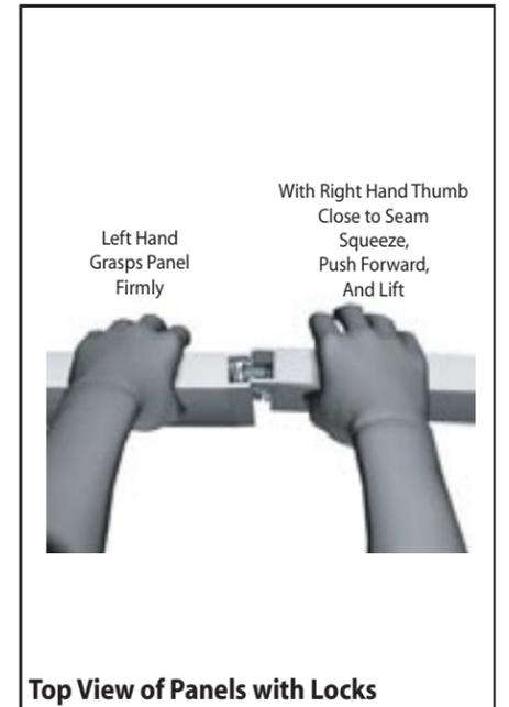
The first level of components contain panel locks that are located at the top of the panel for extra stability and seamless connection. When disassembling panels twist top connection slightly and lift right panel upward.
