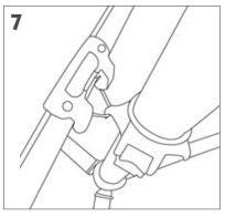
Attach the kicker to the pins to the adjustable ring. The thumbscrew will allow you to adjust the position up or down. The tension between the hanger and kicker maintains the graphic ton the spring stand.
