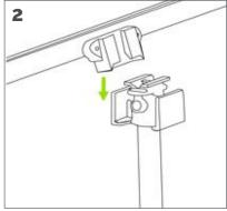
Take the graphic by the hanger and clip it onto the pole head using the center piece.
