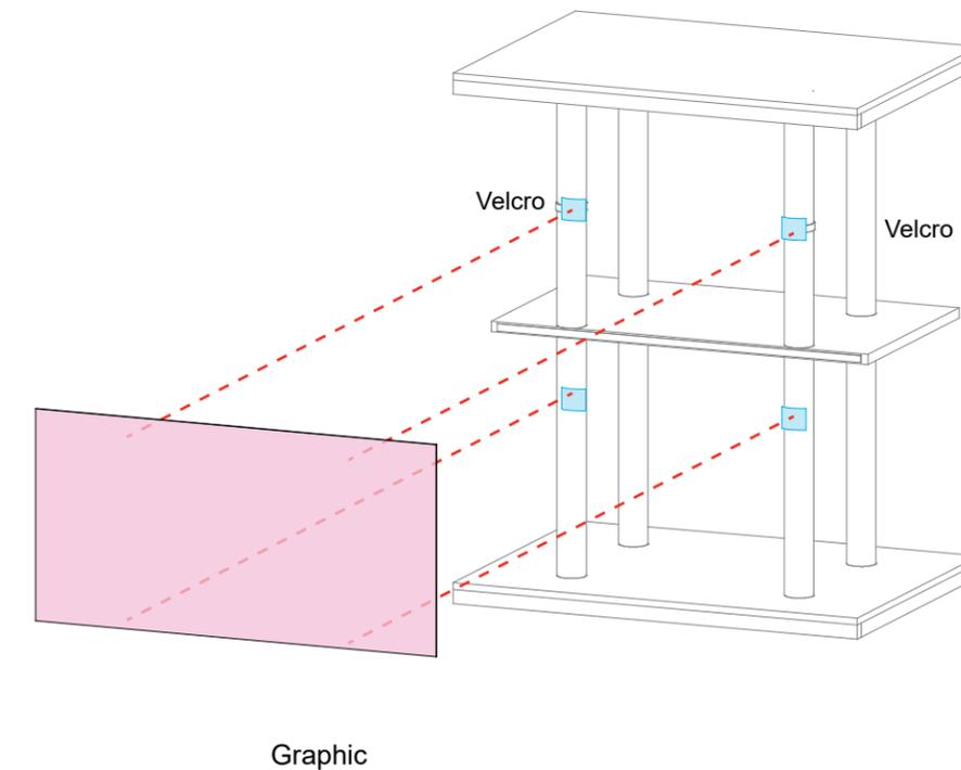
*Note: Velcro must face front of assembled counter.*
