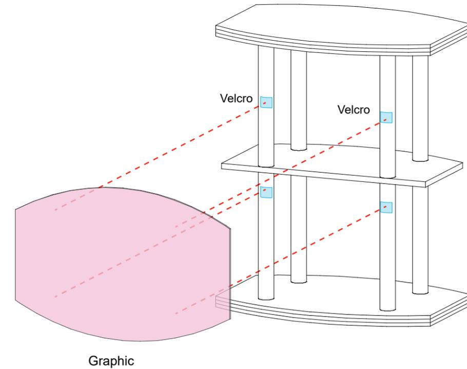
*Note: Velcro must face front of assembled counter.*
