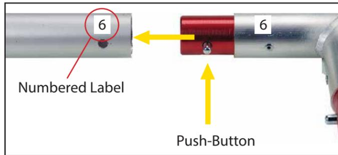
Connections are made by holding the button down and sliding the red tube into opposing tube until button locks into the hole. To disassemble, push button and pull or twist extrusions apart.
