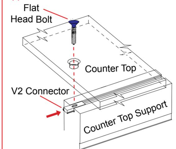
Slide V2 connector into groove of shelf support. Bolt through hole of shelf into threaded hole of V2 connector. Twist Bolt to secure counter top in place.
