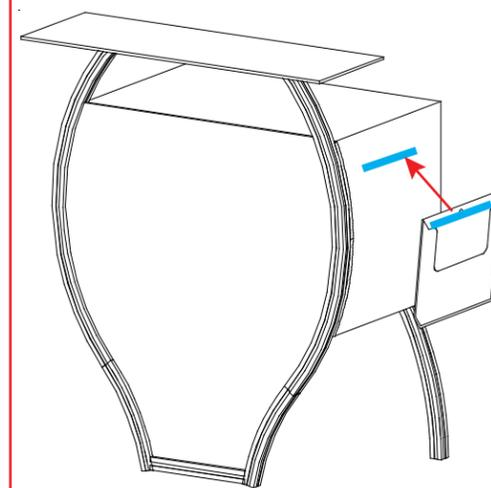
Attach literature pockets with Velcro to sides of pedestal.
