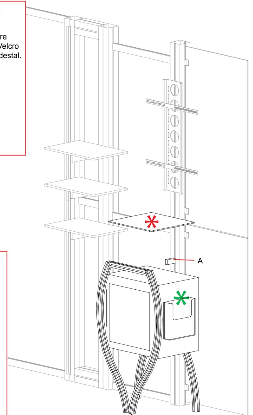
Attach pedestal to mounting connectors in backwall with screwcaps.
