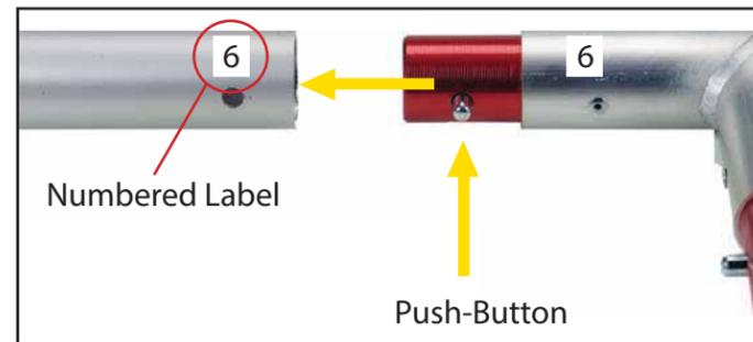
Connections are made by holding the button down and sliding the red tube into opposing tube until button locks into the hole of the opposing tube. To disassemble, push button and pull or twist extrusions apart.
