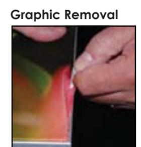
It is important to first insert graphic into each alternater corner then to the sides of the frame. If this is not done, graphic will not fit into the frame correctly.
