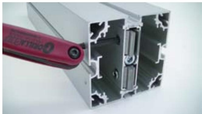
Turn the hex wrench clockwise to open the lock and secure in the groove.
