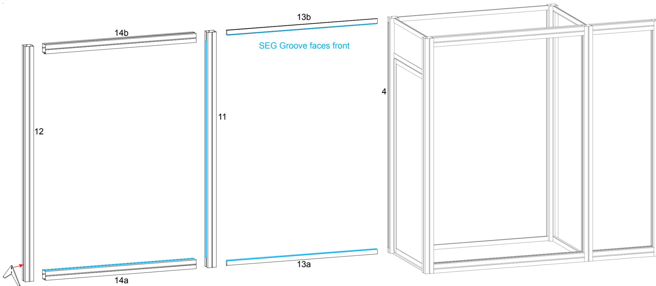
**WHEN DISASSEMBLING ALUMINUM EXTRUSION, TIGHTEN ALL SETSCREWS AND LOCKS TO PREVENT LOSS DURING SHIPPING**
