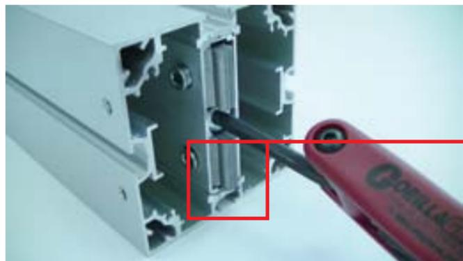
Turn the set screw clockwise to move the lock back into the extrusion, counter-clockwise to move the lock outward.
