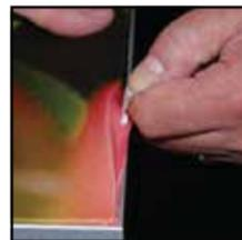
To remove the graphic from the frame, locate the fabric pull tab. Gently pull up on the tab to remove the fabric.
