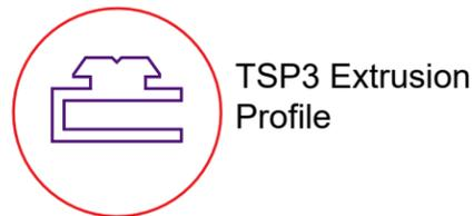
Groove for SEG graphic must face outside of closet assembly.
