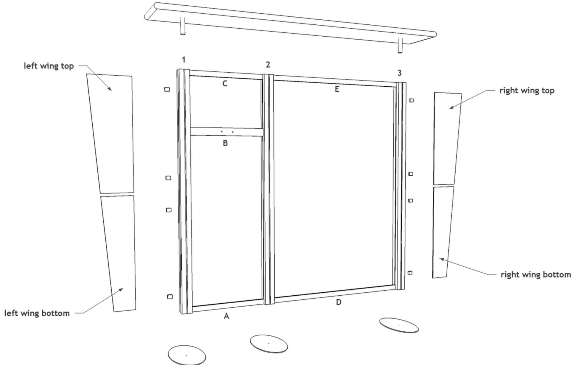
**WHEN DISASSEMBLING ALUMINUM EXTRUSION, TIGHTEN ALL SETSCREWS AND LOCKS TO PREVENT LOSS DURING SHIPPING**
